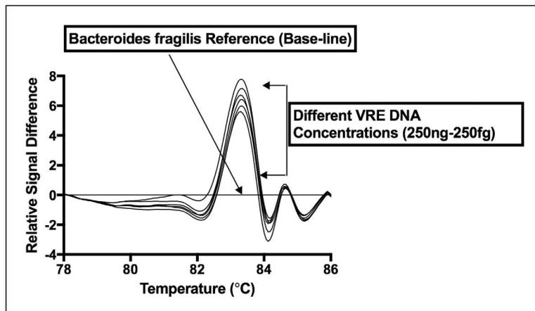
**Figure 4.** Analytical sensitivity of VRE PCR-HRMA assay using the V1 primer set. Data show that the characteristic difference curve shape for VRE (using DNA from VRE *E faecalis* strain ATCC 29212) is maintained over a 6-log concentration range (250 fg to 250 ng DNA).
